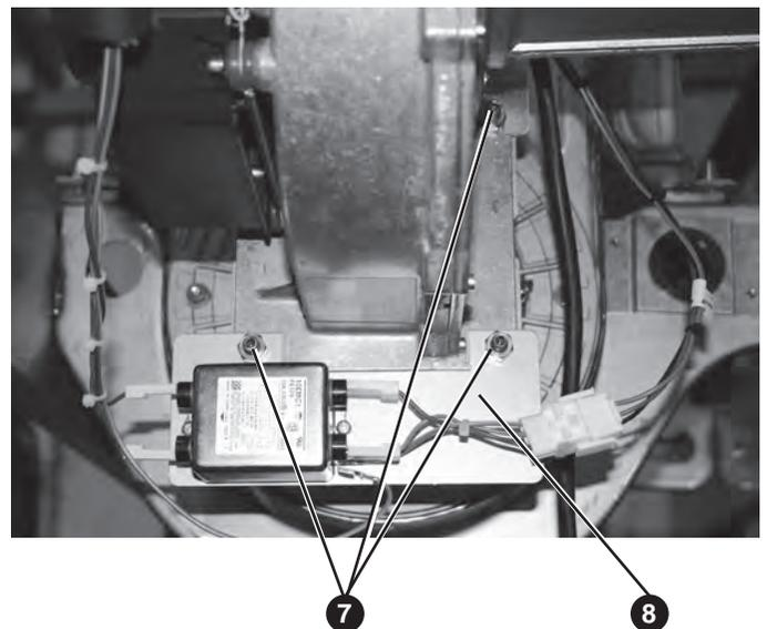
8. Remove the EMC filter bracket.
