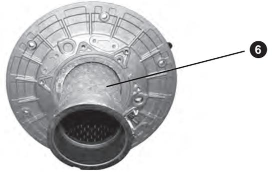
6. Carefully remove the burner, the burner can be cleaned internally only using a soft brush and/or vacuum. The metal fibre outer surface **MUST NOT BE BRUSHED**. If the burner shows signs of damage it must be replaced.
