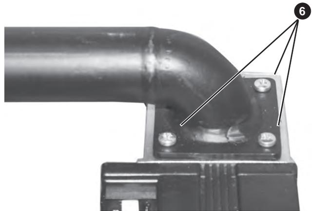
7. Remove the four nuts and washers retaining the fan to the burner mounting plate.
