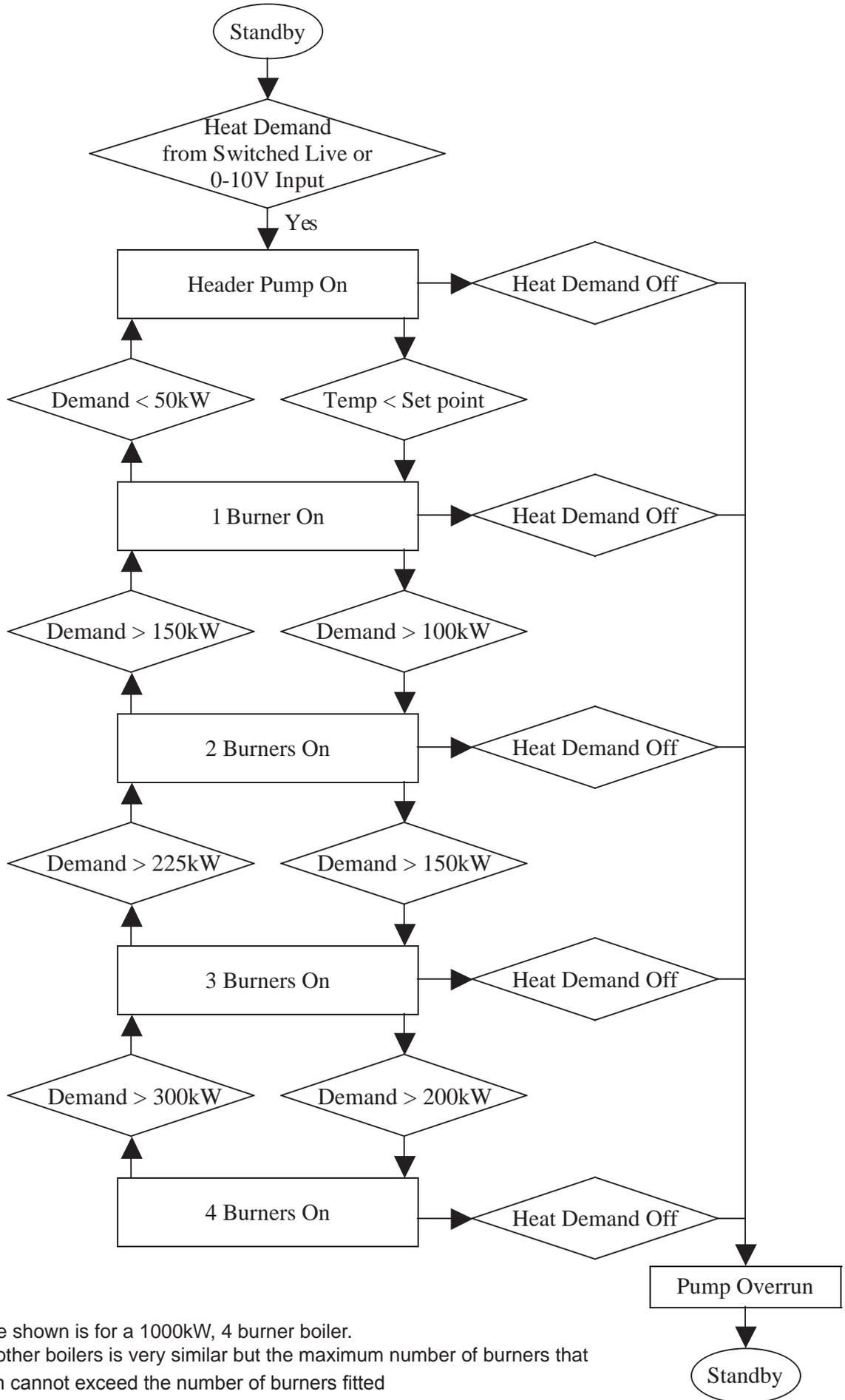
Note: the sequence shown is for a 1000kW, 4 burner boiler. The sequence for other boilers is very similar but the maximum number of burners that can be switched on cannot exceed the number of burners fitted
