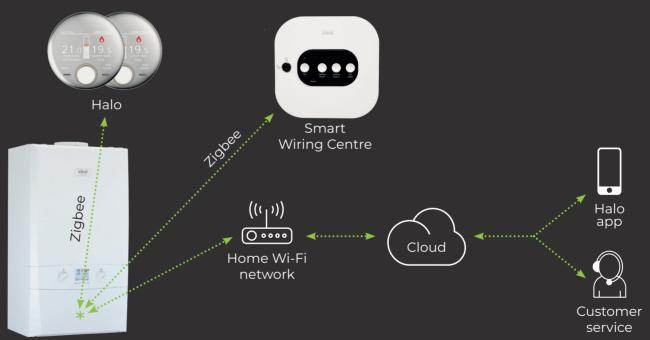
\*Connections via Smart Interface plugged into boiler
