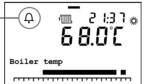
When the fault places the boiler in a safety lockout condition, the fault code and its text are displayed continuously on the screen. Similarly, a small bell appears at the top left of the screen.
