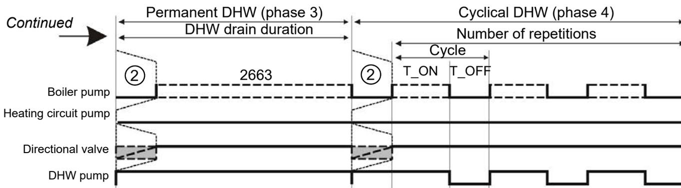
② 3-channel valve after DHW opening time (if the *Directional valve available* is configured).
