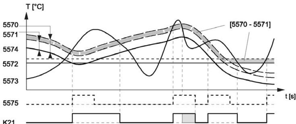
**Assignment or not of the pump/valve kick-start for the K21 and K22 outputs (see parameter 6127):**
