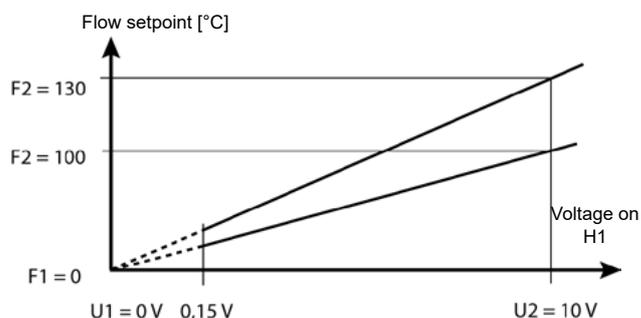
If the input signal goes below the 0.15 V threshold, the heat request is invalidated and therefore not operative.
