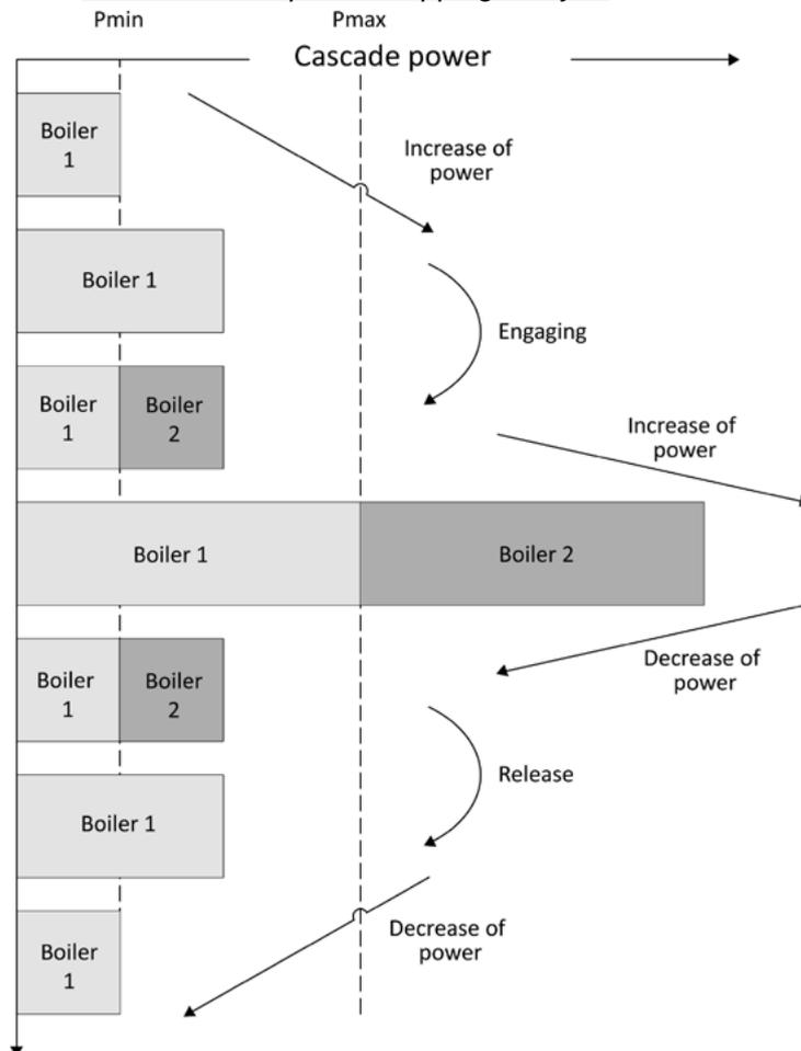
Adjust the power ranges to control the switchovers in the cascade strategies described above. The ranges are common to all the boiler switchovers, these ranges must therefore be adjusted in accordance with the type of boiler in the cascade.
