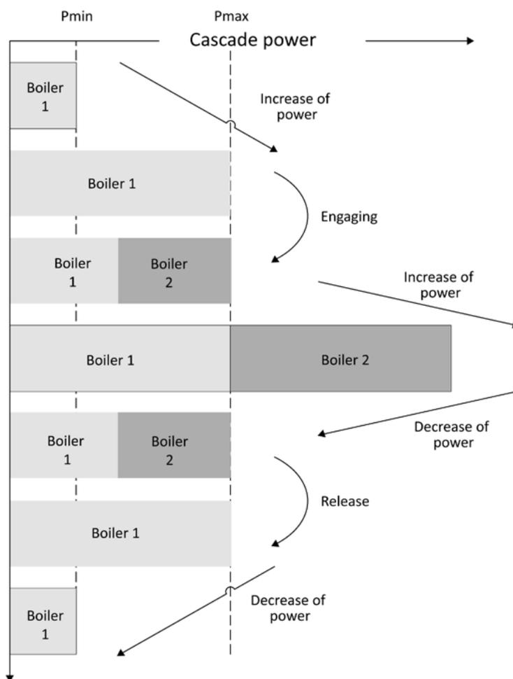
Activation delayed, stopping delayed
