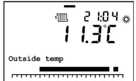
The bottom of the screen is displayed with a scale of 0 to 24 corresponding to the hours of a day. The comfort setpoint request phases are represented by a black square above the scale. The other parts without square correspond to the reduced setpoint requests.
