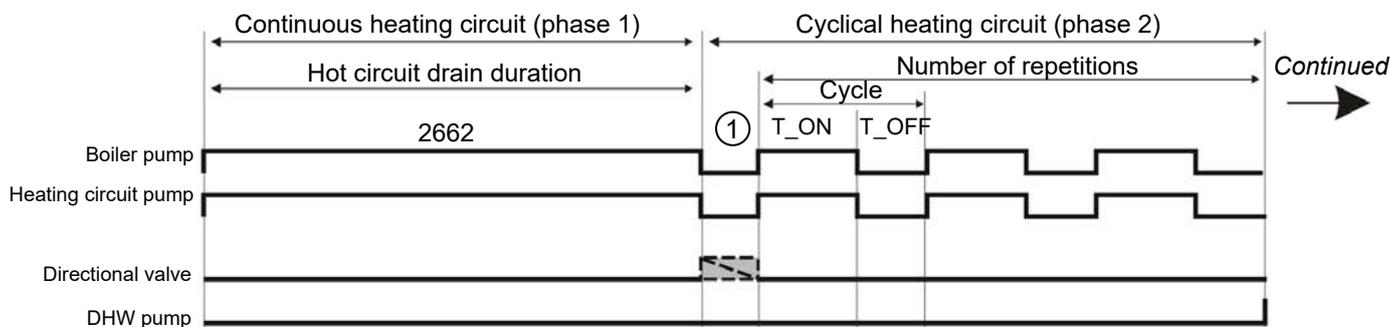
① Mixer heating valve / 3-channel valve opening time
